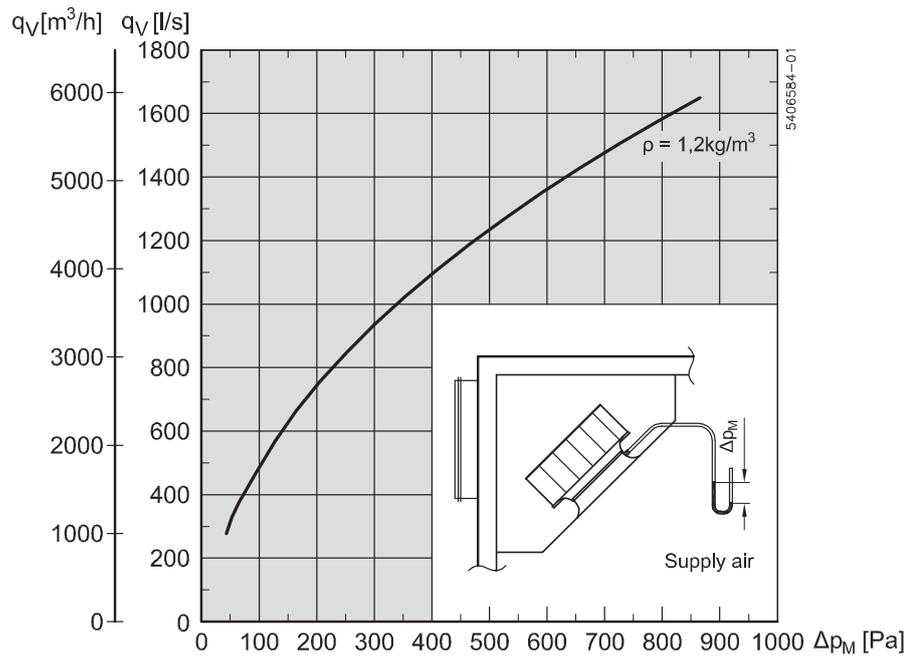
— Airflow ( $q_V$ ) according to pressure difference ( $\Delta p_M$ )
