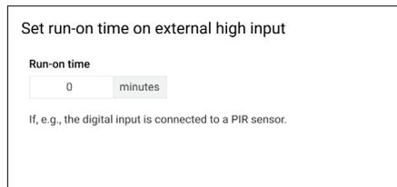
A PIR sensor (motion sensor) can automatically start or increase ventilation from the low speed to the high speed setpoint when there are people present.
