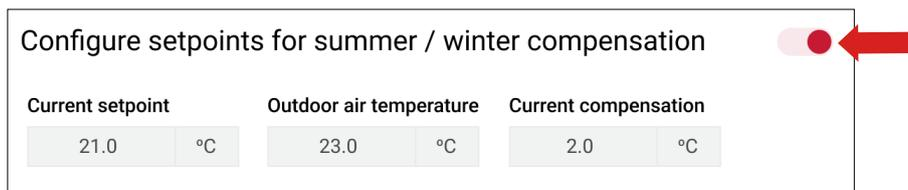
**Summer/winter compensation** can be activated when sliding the round button in the upper right corner to the right. When selected, temperature setpoint compensation offsets will be according to the settings in the **Summer** or **Winter** sections. The difference will be visually reflected in the diagram on the right.
