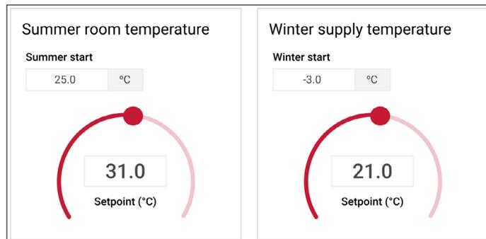
Here you can set the summer **Room temperature setpoint** and the **Summer start** outdoor temperature. In the illustrated example above, the control loop will switch to summer operation when the outdoor air temperature (**Summer start**) reaches 25°C. It will switch back to Winter operation when the outdoor air temperature (**Winter start**) falls to -3°C.
