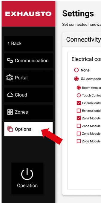
In the **Electrical connection** section under the **Options** settings, you can select optional components to connect to the AHU. Click on **OJ Components** to see a list of available components.
