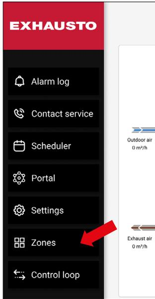
The EXcon+ system supports up to 4 individual zones (4 room controllers). The Zones section is only shown if one or more room controllers have been connected. If you click the **Zones** button in the lower-left corner of the main menu, you will see the following screen:
