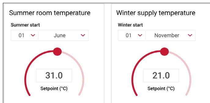
With a calendar-triggered changeover between summer and winter operation, you must choose a specific date for the changeover. In this case the outdoor air temperatures will have no influence on the timing for the changeover.
