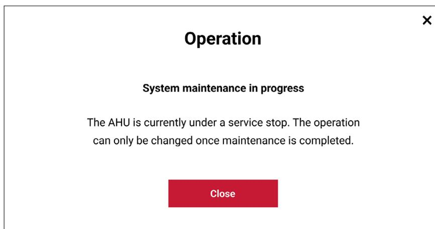
**Service stop** can only be activated/deactivated from the operation panel located on the Air Handling Unit, or if your login device has a cable connection to the AHU. Remote access will not be able to start the Air Handling Unit.
