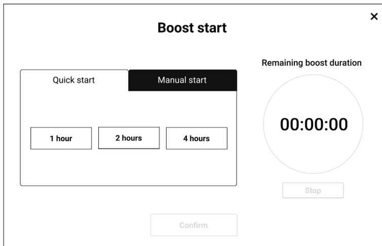
A boost is a way to increase the airflow and pressure, so you quickly achieve the desired temperature and air quality. Under the **Quick Start** tab (see above), you can run a boost for either 1, 2, or 4 hours. Once you have clicked on one of these buttons, a count-down timer is displayed on the right side of the screen. This timer tells you exactly how much time remains before the boost operation has finished.
