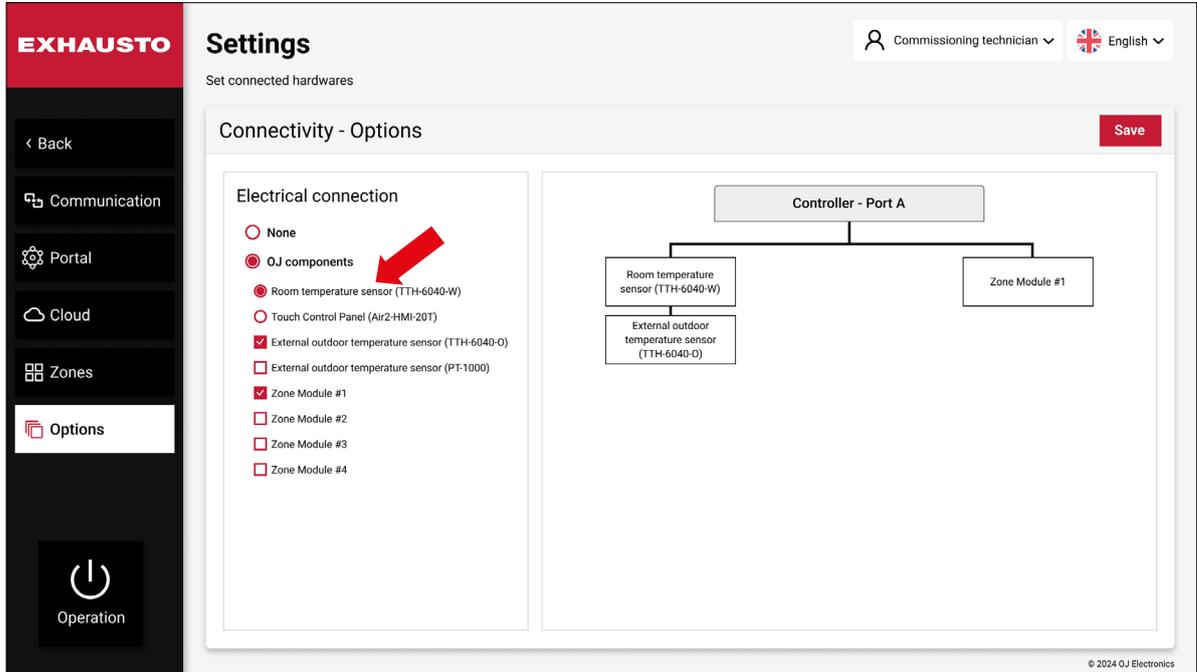
Physically, the external Modbus components must be connected to the **RS485** port A on the controller. These settings are used for connecting components supported by OJ Electronics, for example, room temperature sensors, 2-inch touch control panels, external outdoor temperature sensors, and zone modules. For ease of overview, the connection diagram is illustrated graphically to the right. This may come in handy when you are working on rather complex AHUs.
