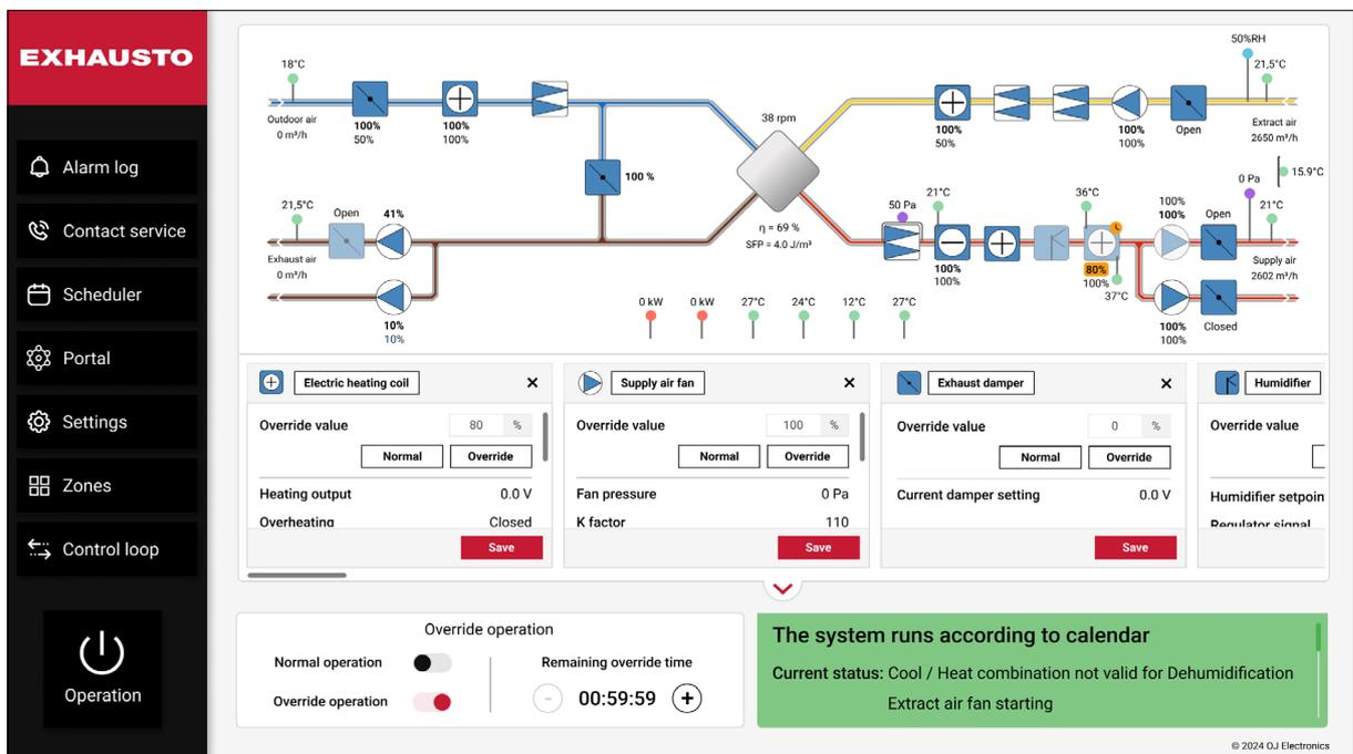
This ability is particularly useful if you need to monitor and compare data from various components. The visual status information and the detailed component data offer you the ability to perform a quick analysis of the system's performance. It is recommended to use this screen as the central information tool. Here, you immediately become aware of the system status. This enables you to quickly identify any required corrective actions.
