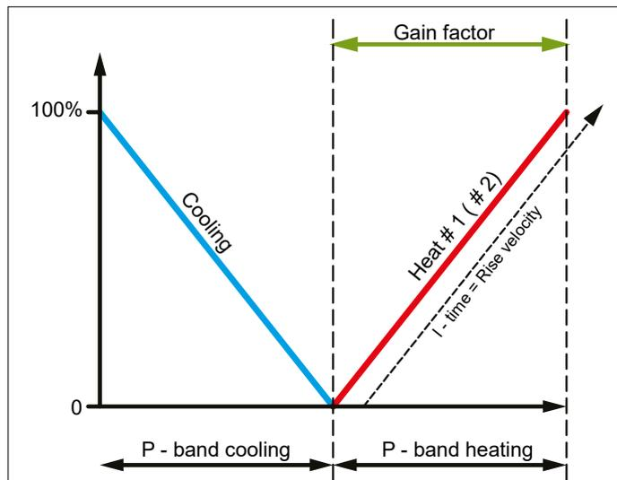
The control loop uses half of the error signal as a “here-and-now-reaction” (P-band) and the output slope is influenced by the integral signal (I-time).
