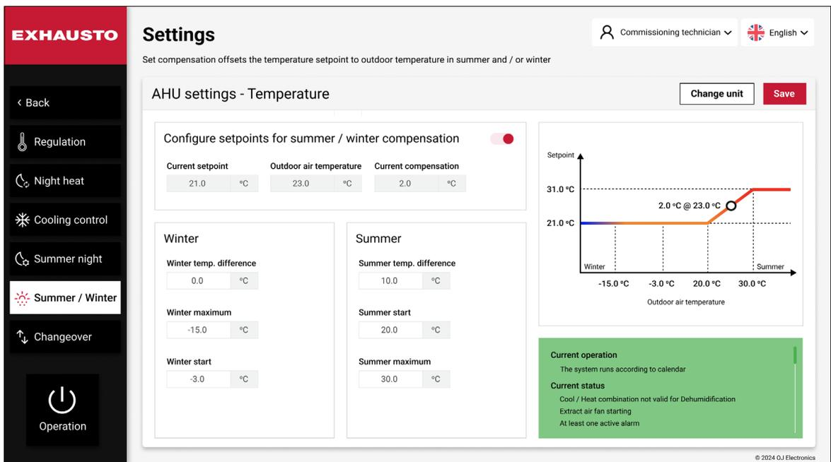
The Summer/Winter compensation adds an offset to the temperature setpoint depending on the current Outdoor temperature.
