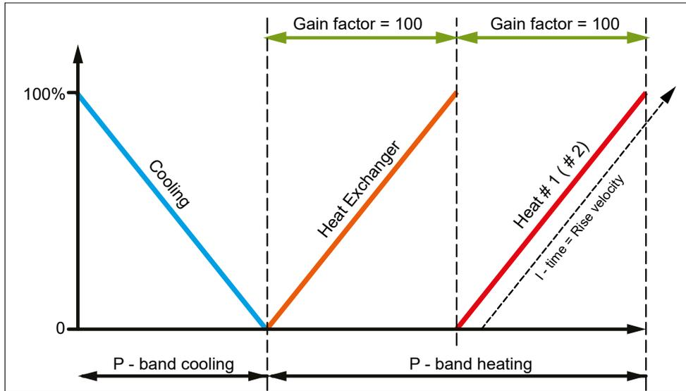
In the example below, the Gain factor setting supports a two times higher heating power from Heat#1 than from the Heat exchanger.
