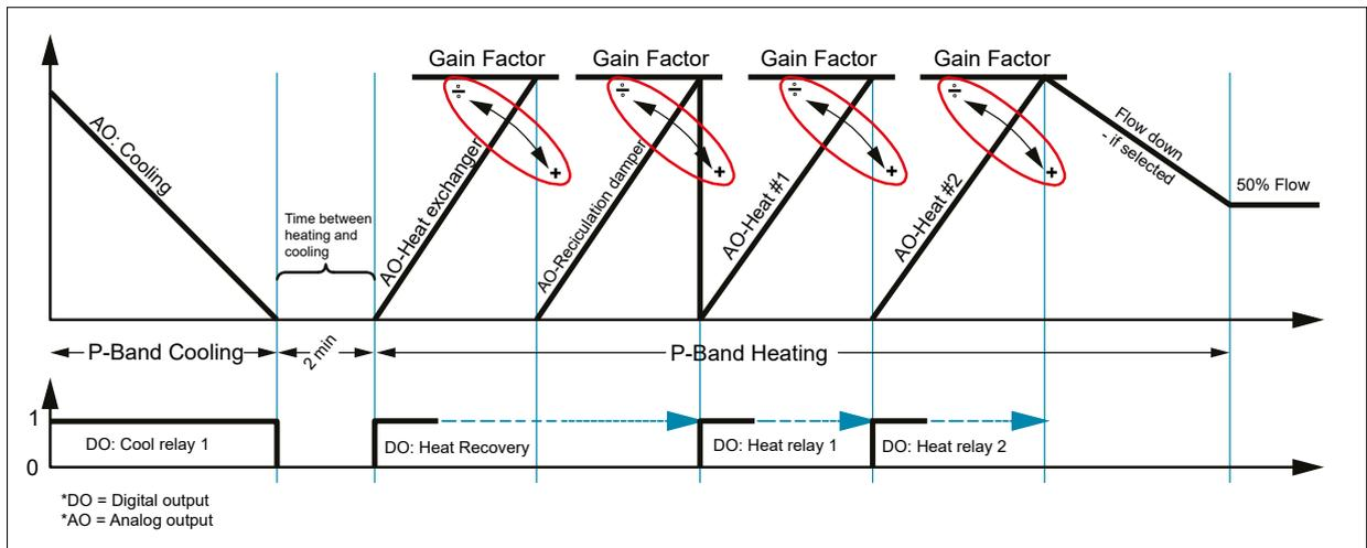
The control sequence has a two-minute switching delay between heating and cooling mode.
