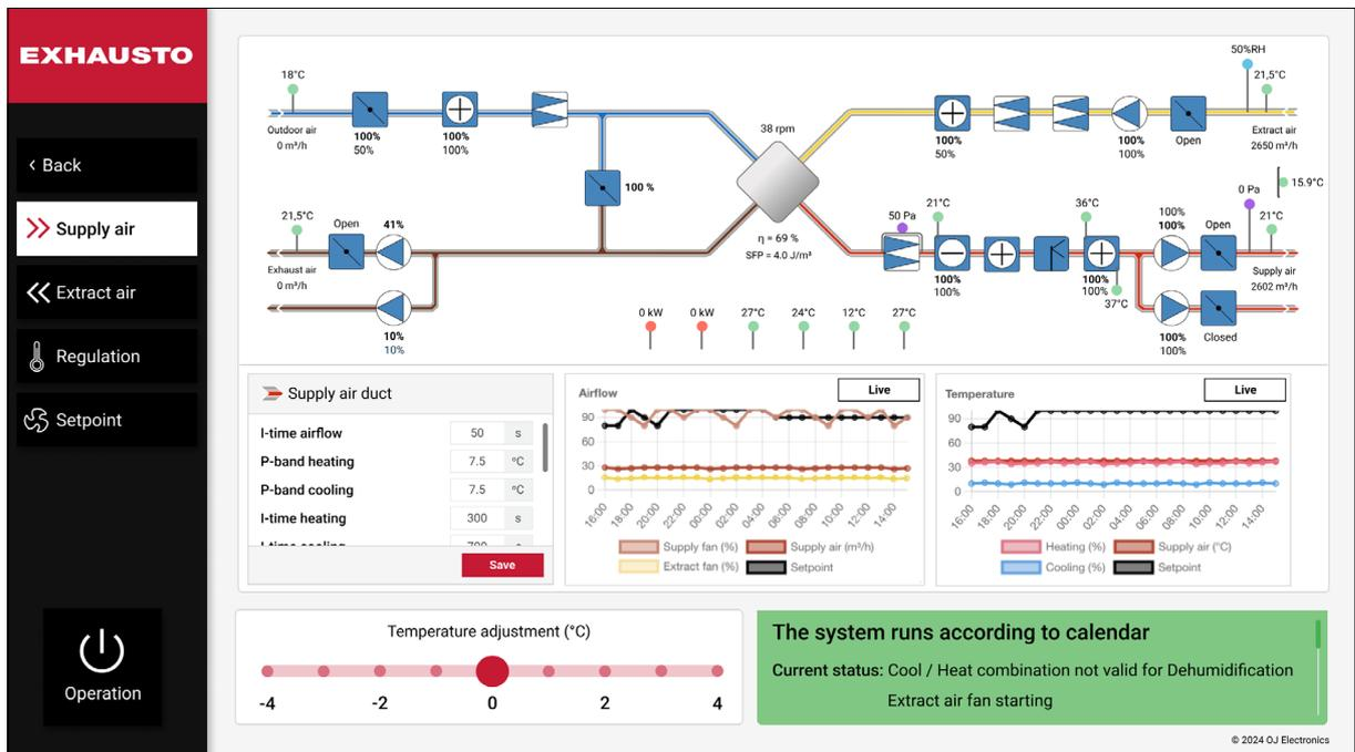
Here you can set and finetune the control loops. First, you need to complete the fan settings and then you can proceed to the temperature settings. Note, that you will need to complete the supply air temperature settings before the extract air temperature settings.
