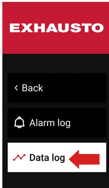
The **Data log** is a useful diagnostic tool that gives you a visual representation of selected climate and AHU parameters over time. You can choose between climate parameters (**Climate chart selector**) and other parameters (**AHU chart selector**). These parameters can be displayed over time in a chart.
