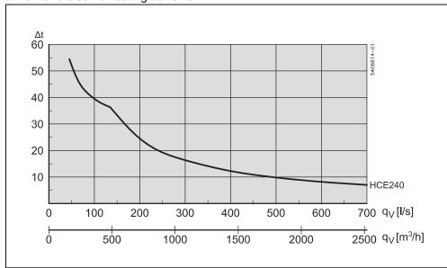
Pressure drop across electric heating coil
