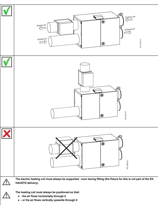
Take note of the air direction (see the air-direction arrow on the electric heating coil door).
