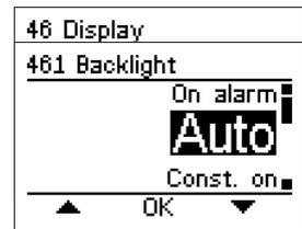
Use the **◀** and **▶** buttons to navigate through the menu to **Backlight** and press the **OK** button.
