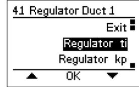
The  $T_i$  factor can then be set in the range 1–4000 seconds with a factory setting of 100 seconds.
