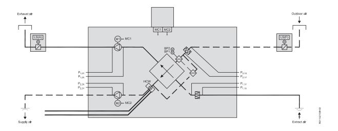
The simplified diagram shows a VEX unit with LEFT fan placement.
