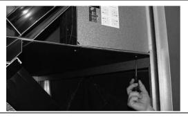
Fit the box with the frequency converter and secure with screws.
