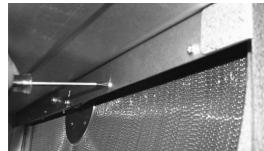
Remove the bracket with the sealing strip closest to the service door.
