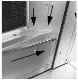
To seal the blowout zone, apply sealant to the rotor shaft and around the door as shown in the picture.
