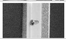
Use screws to fit the sealing strip to the blowout zone. Wait until the blowout zone is fitted by the rotor, and the distance between the rotor and brushes is adjusted correctly before finally tightening the sealing strip.
