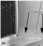
To seal the blowout zone, apply sealant to the rotor shaft and around the door as shown in the picture.
