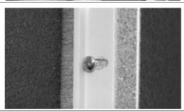
Use screws to fit the sealing strip to the blowout zone. Wait until the blowout zone is fitted at the rotor and the distance between the rotor and brushes is adjusted correctly, before finally tightening the sealing strip.
