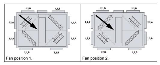
The trim damper must be fitted either in the outdoor air intake or the extraction intake depending on the measured pressure conditions. See Section 3.2 commissioning section.
