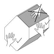
The counter flow heat exchanger can be removed from both sides of the unit. Choosing the side that is opposite the connection box on top of the unit avoids having to remove the bypass damper.
