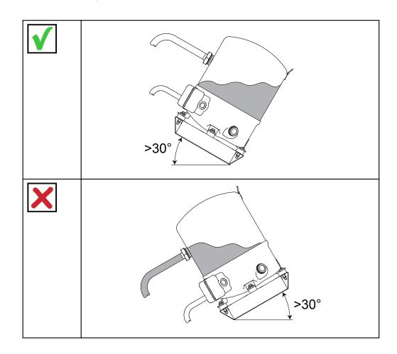
Lifting with forklift truck
