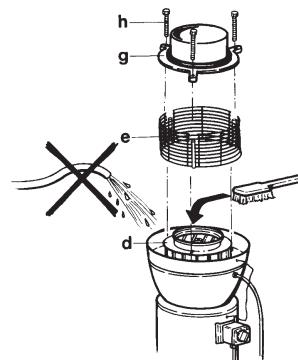
**Do not** flush the fan with water while it stands in this position.
