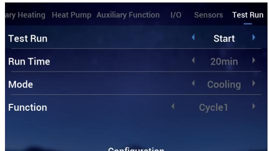
A screenshot of the same control panel showing the 'Test Run' configuration screen after changes. The 'Start' button is now highlighted. The 'Run Time' is set to 20min, 'Mode' is Cooling, and 'Function' is Cycle1. A yellow arrow points from the first screen to the second, indicating the transition. |
