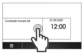
To start the controller, press anywhere on the screen with the words "Controller turned off", then appears the message "Active controller?". Confirm the message.
