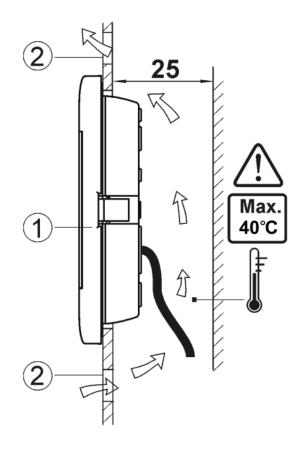
Control panel mounting requirements. 1 – control panel, 2 – vent holes to provide air circulation.
