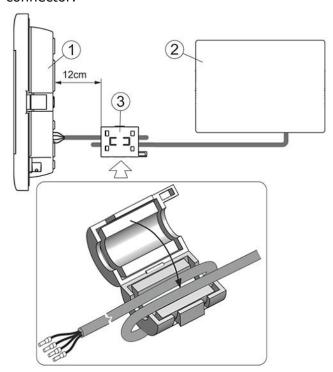
Installation EMC filter: 1 - control panel, 2 - TAC5/TAC6 controller module, 3 - EMC filter (type ZCAT1518-073).
