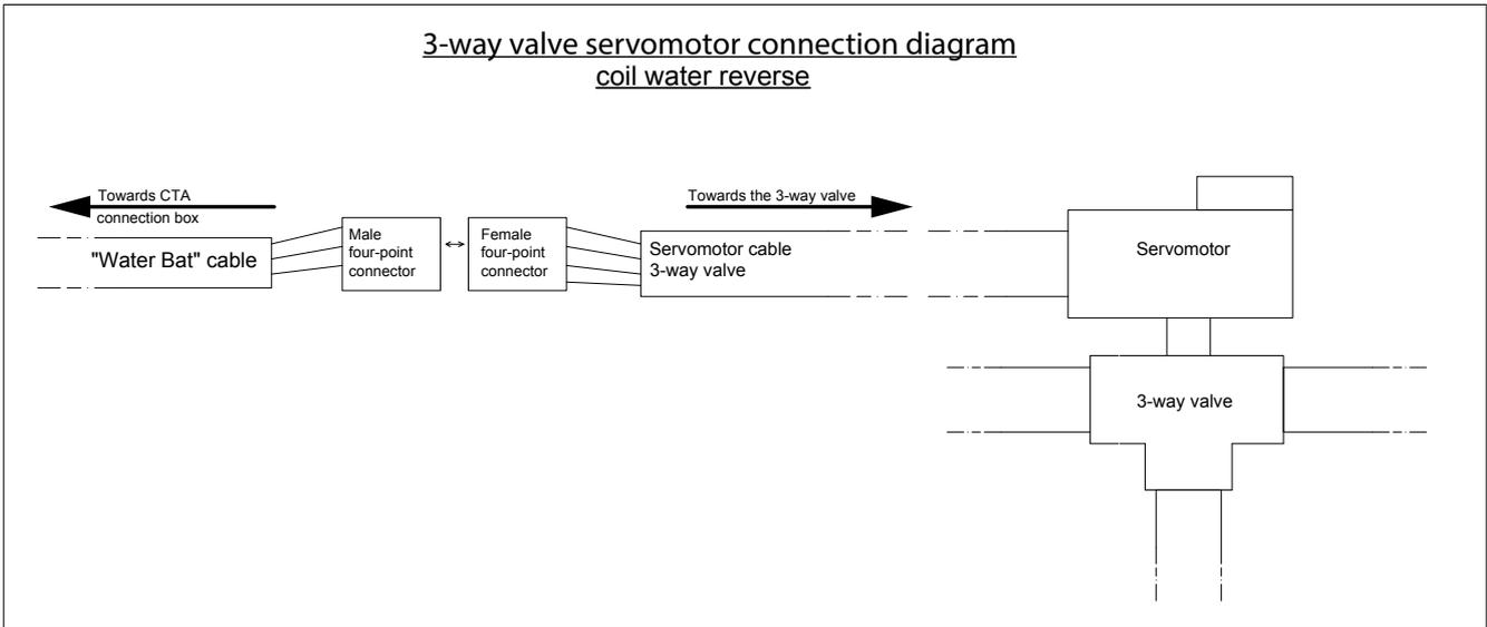
Position the temperature probe in the 3-way valve on the internal coil, reverse water flow side, with a plastic collar. To increase the accuracy of the fluid temperature measurement, isolate the probe and the 3-way valve (see wiring diagram below)
