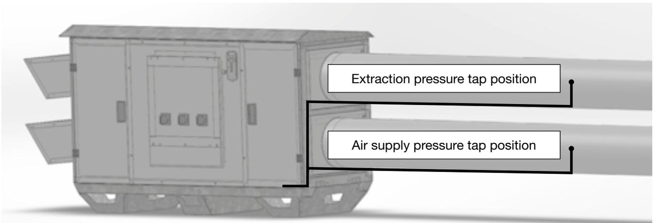
**Caution:** to obtain more accurate measurements, the pressure must be measured where there is the least risk of turbulence, i.e. on a straight section of the duct. The minimum distance to be respected from any disturbance is at least twice the diagonal of a rectangular section and at least twice the diameter of a circular section.
