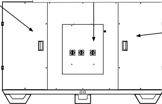
The unit's rating plate is duplicated. One plate is located on the back of the quick access hatch and another on the side panel.
