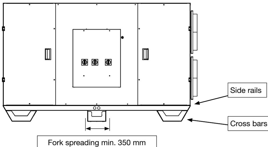
Handling with slings: use handling bars placed in the cross bars. The rigidity at the sag of bars must be adapted to the weight of the crate. Place the sling buckles around the handling bars and place spreaders above the unit to avoid damaging the structure. See diagram below. mounted. See Section 0 for the fitting of accessories.
