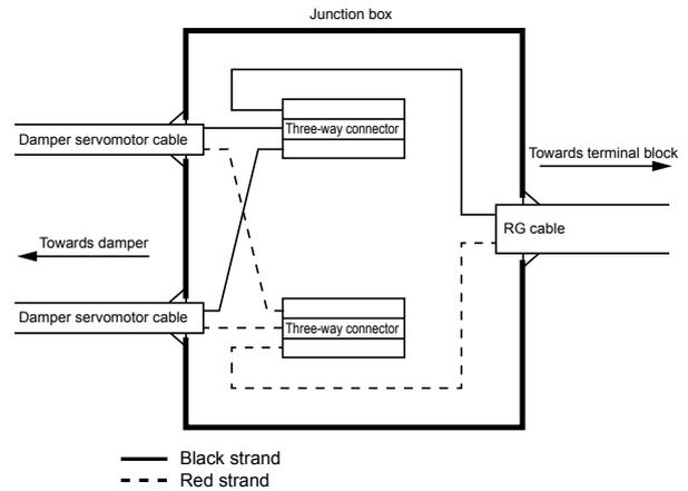
Once this wiring has been completed, shut-off damper side, wire the equipment electronic board side.
