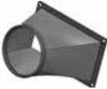
The flexible sleeve is a layer of glass fibre, fire class M0, supplied with four screws M8, eight washers and four nuts. This sleeve can be fixed to a damper or directly to the opening frames. See Section 3.4. for sleeve dimensions.
