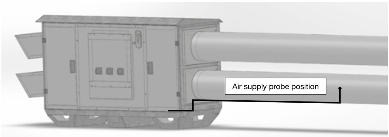
**Caution:** When the system has a hot (water or electric), cold or changeover coil, the probe must be positioned at least 1.5 metres after these heating components - to guarantee a uniform temperature in the section.
