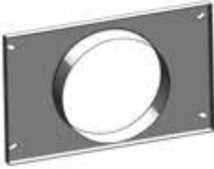
The adapters are supplied with four screws M8 to install them on the unit. Glue the seal 10x20, supplied with the unit, to the connection between the inserts M8 and the opening to keep the unit leaktight (air and water) between the adapter and the unit. Then screw each adapter into the frame inserts. Circular ducts must be fitted with a seal to connect them. See the diameters per machine in Section 3.3.
