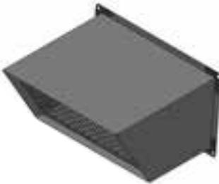
The hoods are supplied with screws M8 and a self-adhesive seal of section 10/20 mm in EPDM. Glue the seal to the hood flange to keep the structure leaktight.
